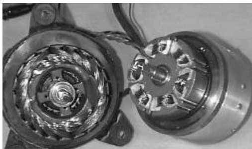
Fig. 12. Comparative analysis of the Copper volume of the endwindings in the armature of a conventional Brush DC motor with a lap winding and the SMC stator of a Brushless DC motor with concentrated winding (same application and specifications)
