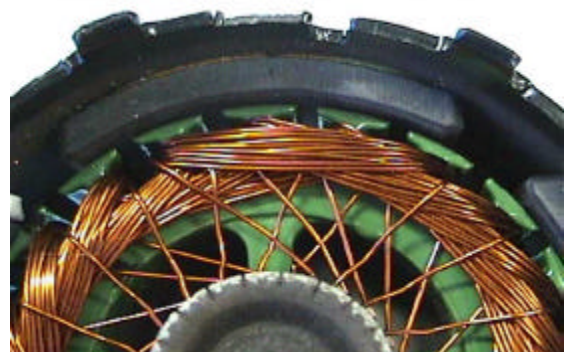
Fig. 8. SMC Armature of a Brush DC motor for an automotive application (concentrated winding and axially inserted end-windings)
