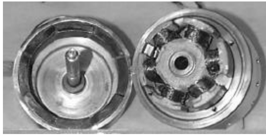
Fig. 10. Brushless DC motor for an automotive electric fan (stator with concentrated winding, yoke made of SMC)
