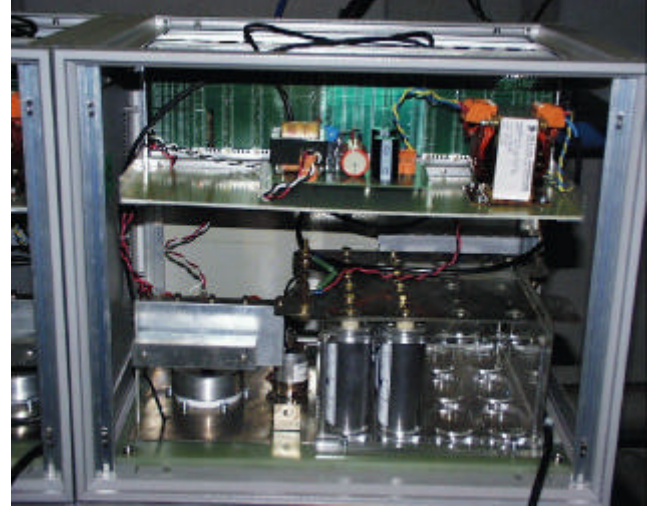
Fig. 3: Assembly of one of the septum pulsers.
