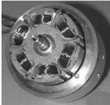
Fig. 11. SMC stator of a Brushless DC motor for an automotive electric fan (concentrated winding, irregular distribution of slots)
