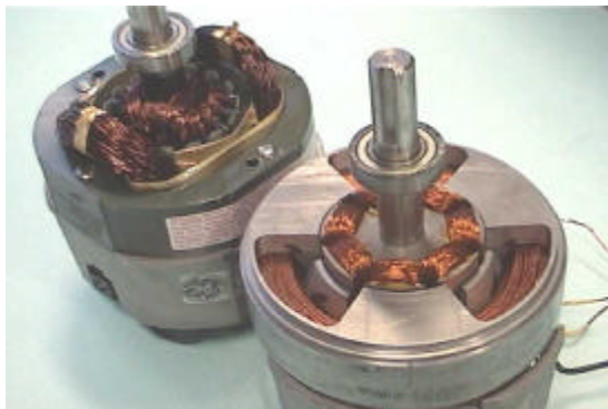
Fig. 9. SMC prototype and conventional universal motor
