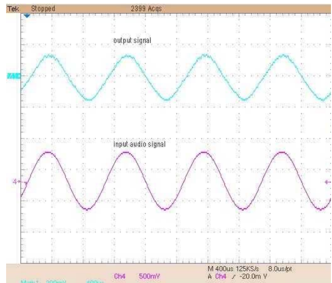
Fig. 7. Experimental waveforms for the output stage
