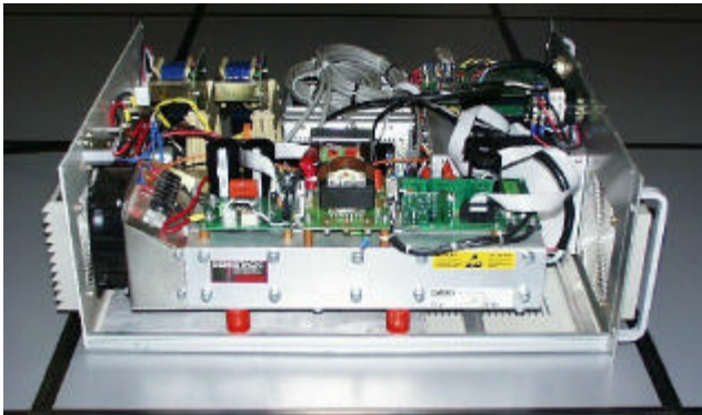
Fig. 5: internal assembly of the quadrupole power supply
