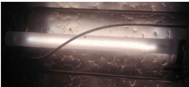
Fig. 9 – Discharge Picture – Resonance at 52kHz.
