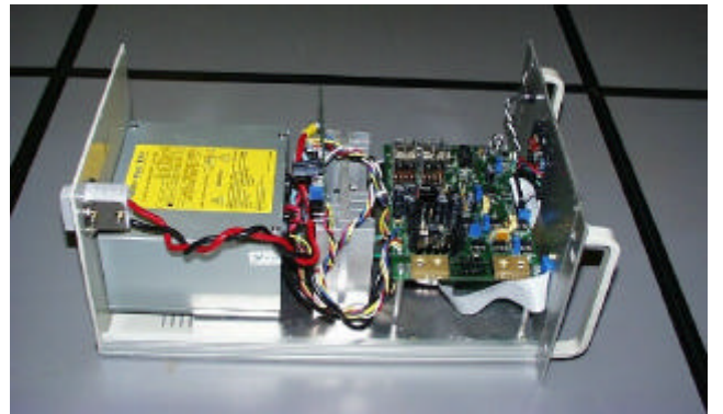
Fig. 3: Corrector power supply internal assembly.
