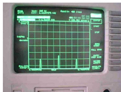
(a) Detail of the components generated by the switching frequency in the phase a current, to 1200 rpm (60 Hz).
