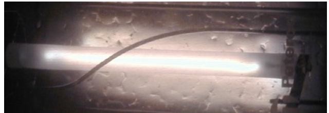
Fig. 10 – Discharge Picture – Resonance at 48kHz.
