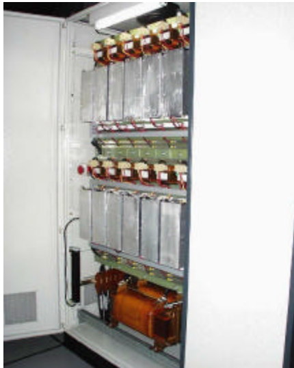
Fig. 11: Rear view assembly of the 12-dipole booster power supply showing the 12-SMPS modules.
