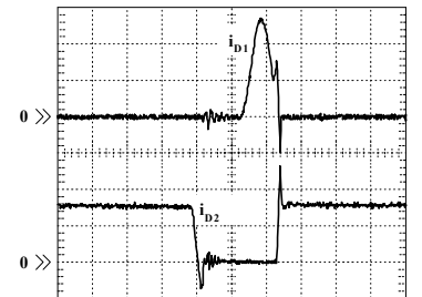
i_{D1} : 5A/div; 2μs/div i_{D2} : 5A/div; 2μs/div (f) Diodes D_1 e D_2 , V_{in}(\omega t) \approx V_{in(pk)}
