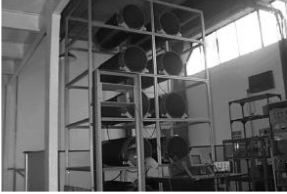
Fig. 1. The pulse generator structure.
