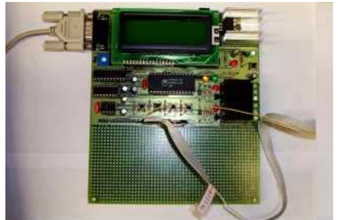
Figure 4: Circuit of Control based on the microcontroller AT89C52.
