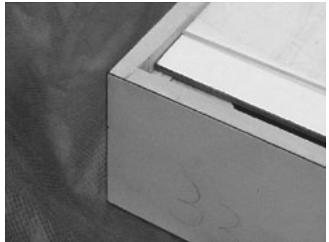
Figure 1 – Box border photo showing the height lowering, the white panel base, and the PET panel covering. The Formica covering of the sides can also be seen.
