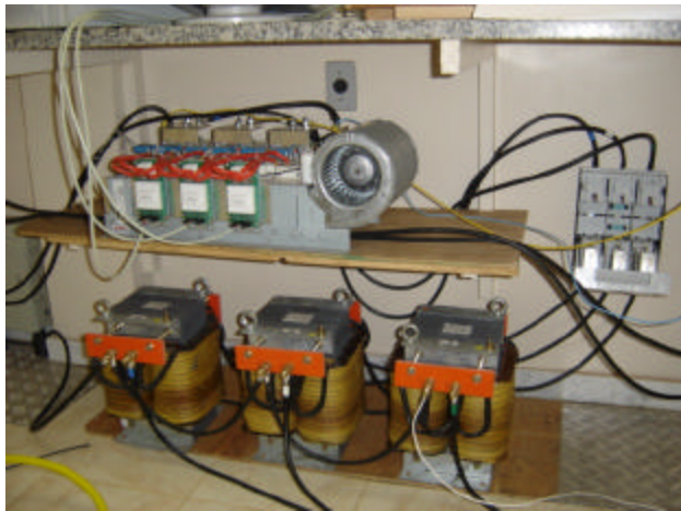
Fig. 12: Picture of one VSC and its transformers bank.
