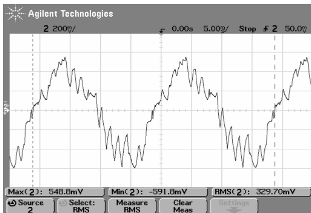
Fig. 16. Three-level inverter: experimental output line current with \mu = 0 or 1 and m = 0.9 (Vert.: 2A/div; Hor.: 5ms/div).
