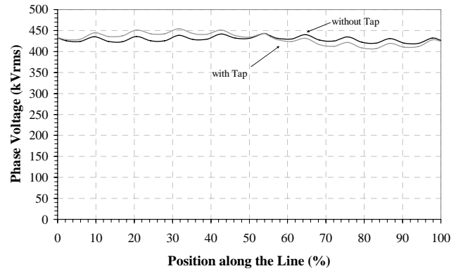
Fig. 14. Voltage profile with a 100 MW shunt tap.
