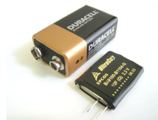
Fig. 3: Typical available supercapacitor cell of 10F/2.3V.
