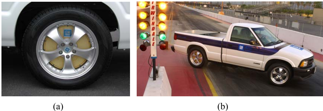
Figure 8. GM's wheel hub motor (a) being mounted on a S-10 demonstration vehicle (b).
