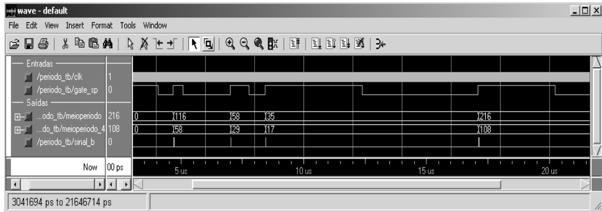
Fig 5 - Simulation results of VHDL behavior, description of component PERIOD.
