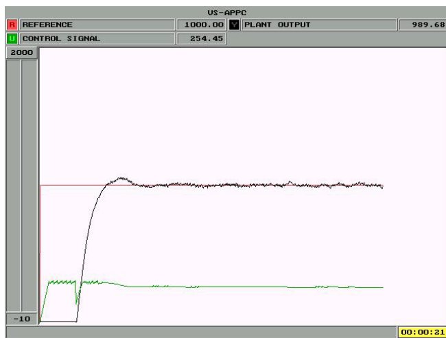
Fig. 6. Experimental result 1: VS-APPC for a speed control of a three-phase induction motor.
