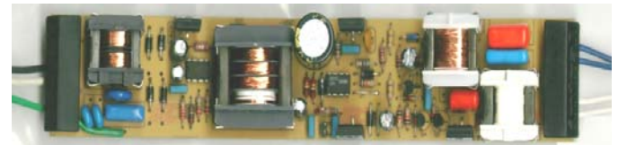
Fig. 12. Prototype of the proposed electronic ballast.
