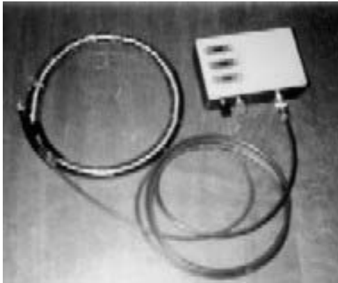
Fig. 6. View of the Rogowski Coil and the Integrator.
