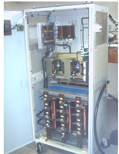
Fig. 10 10 kVA experimental setup of the input stage of Fig. 1 (b). Three-phase transformer, input inductors, interphase transformer and 12-pulse diode rectifier
