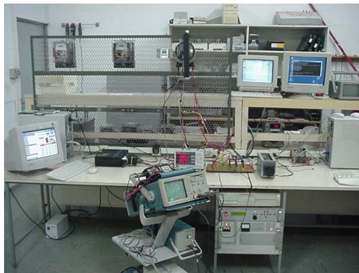
Figure 2 – General view of experimental set-up for meter tests.
