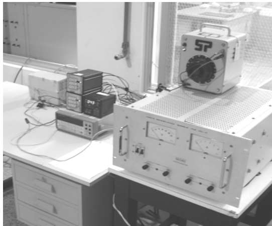
Fig. 3. Test apparatus for the performed tests of the auto-transformer.
