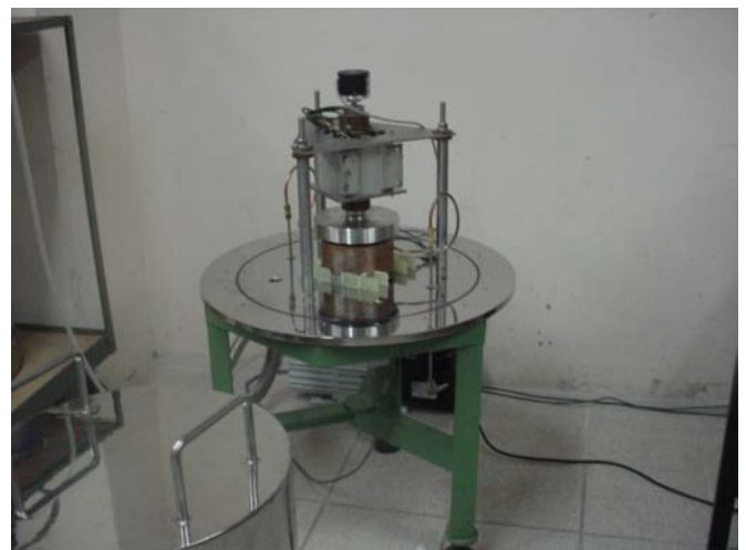
Fig. 2. Flywheel prototype photograph showing (from up to down): the encoder, SR drive, flywheel and SMB rotor, SMB stator and vacuum chamber.
