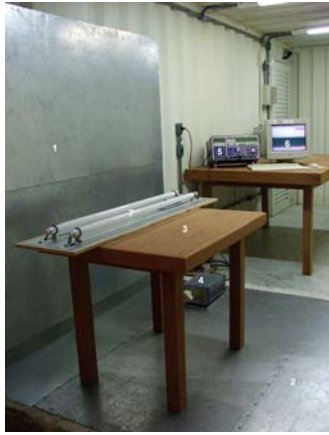
Fig. 2. Configuration for disturbance voltage tests (MagLab/EEL/UFSC).
