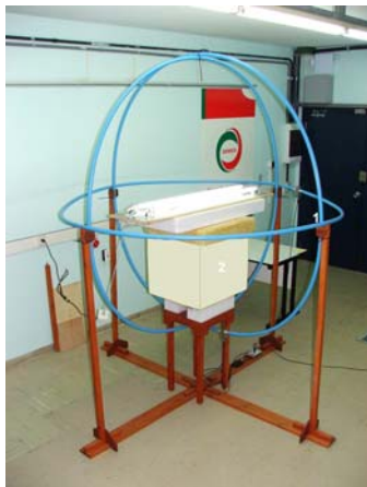
Fig. 3. Configuration for radiated disturbance tests (MagLab/EEL/UFSC).
