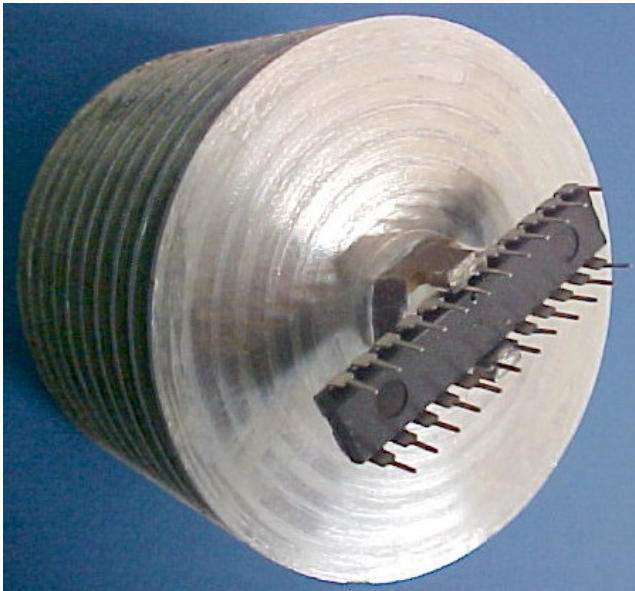
Fig. 6. Heatsink developed for L6208N.
