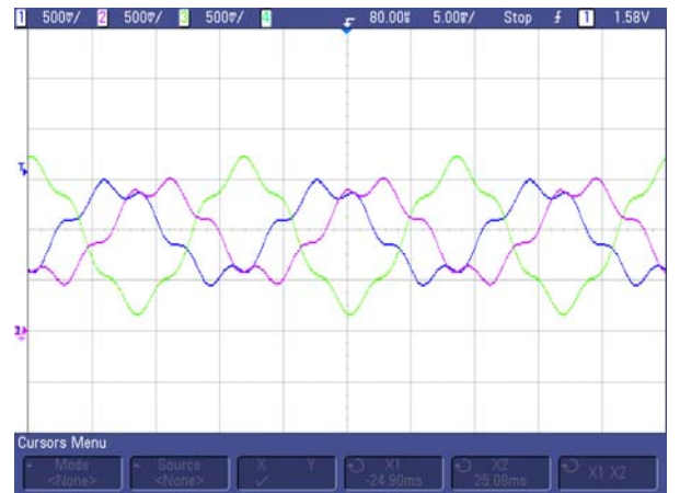
Fig. 8. Case C generated voltage with positive sequence (1 p.u.), negative sequence (0.35 p.u.) and 5 th (0.2 p.u.). Phase R (green), phase S (blue) and phase T (magenta). Scales: 0.5 V/div and 5 ms/div.
