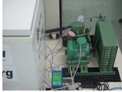
(b) Details – Temperature and Pressure Sensors
