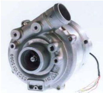
Fig. 4. eBooster from BorgWarner – an electrically power air compressor providing pressurized air for the support of the turbocharger at low engine speeds [18].
