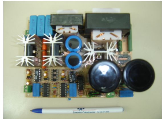
Fig. 8: Photograph of the high voltage circuit prototype.
