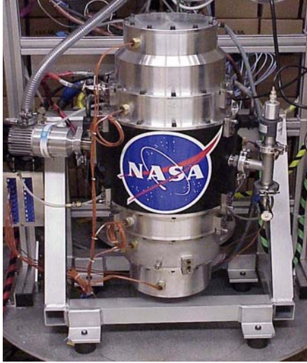
Fig. 7. NASA G2 flywheel for attitude control and energy storage (night-day). 40 000 rpm, 3 kW motor/generator [25].
