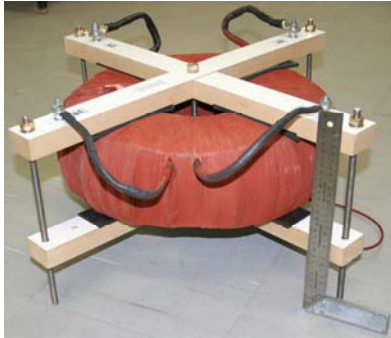
Fig. 11. Developed 1 kHz 50 kW toroidal transformer.
