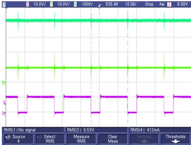
Fig. 8 Voltage source connected to a series resistance - 25 \Omega load – load voltage (light green - above), load current (dark green - middle), MOSFET drain voltage (cyan - below).
